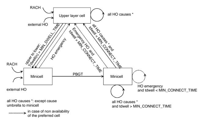
Figure C.7: Complete handover diagram for minicells
