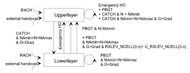
Figure D.6: Handovers in case of availability of the target cell
