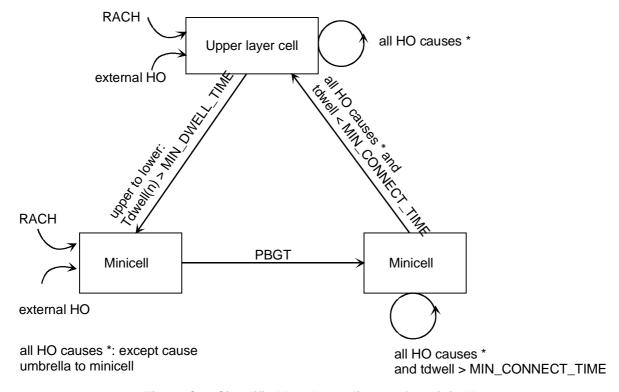
Figure C.6: Simplified handover diagram for minicells
