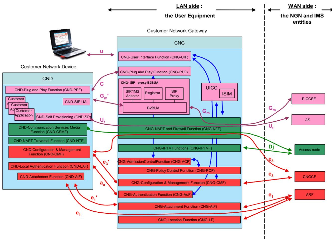
Figure 4.5: SIP IETF CND connected to the NGN-IMS network through a CNG
