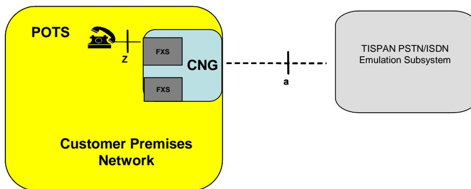
**Figure 4.4: Non-IP devices connected to the NGN network through a CNG (PES scenario)**
