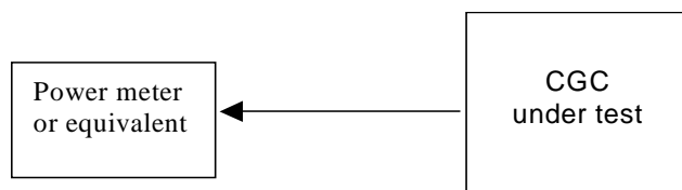
Figure D.1: Measuring system Set-up for maximum output power, total power dynamic range
