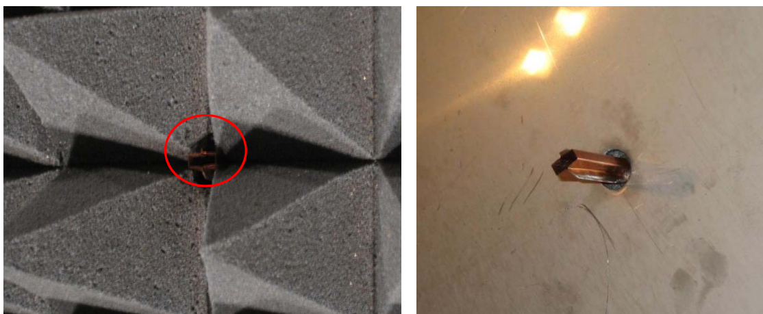
Figure 3: Left: Horn antenna fitted in pyramidal absorbers; Right: Horn antenna protruding the centre of the metal plate
