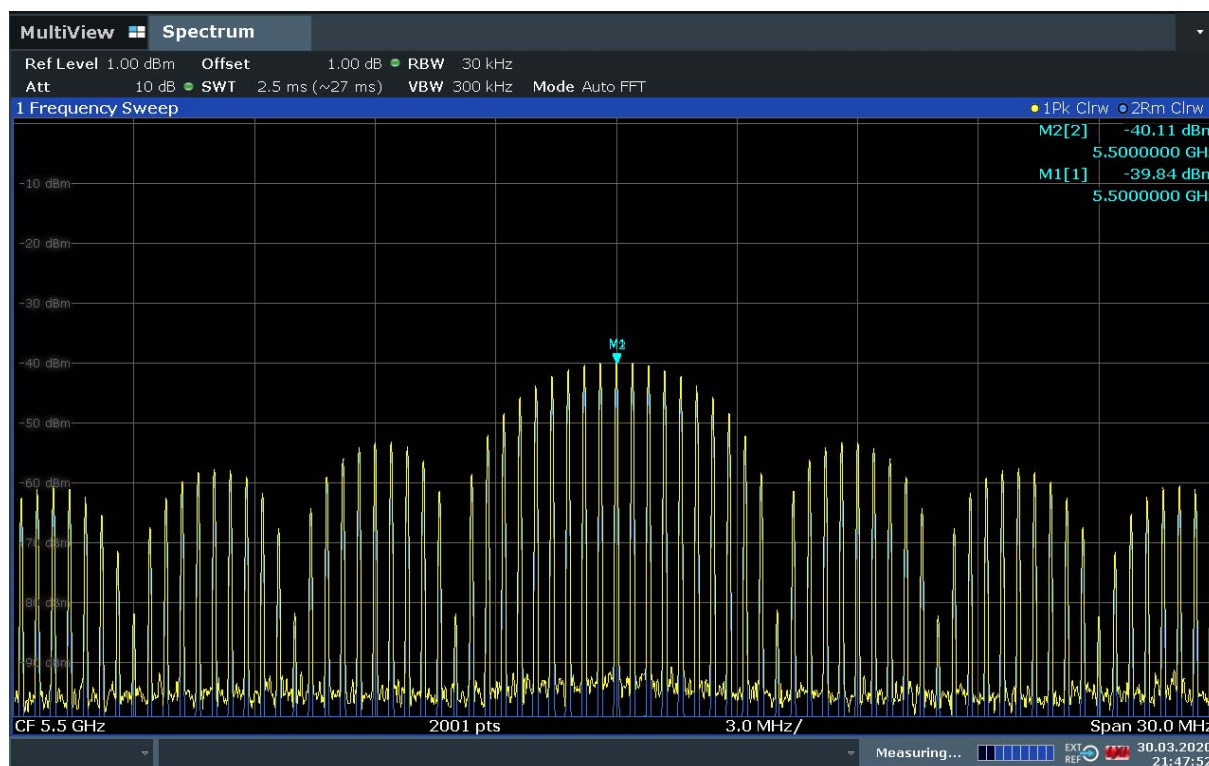
Figure F.6: Max and mean PSD of a pulse train line spectrum
