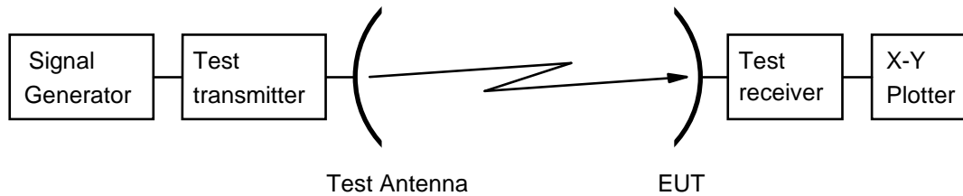
Figure 9: Test arrangement - antenna transmit radiation pattern measurement
