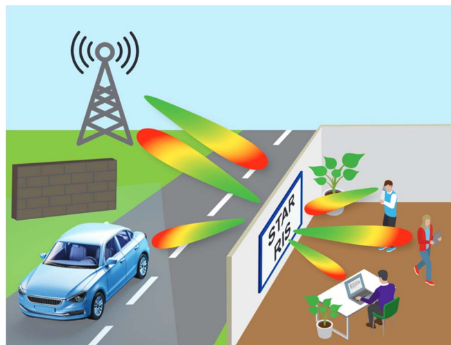
Figure 5.5-1: STAR-RIS indoor to outdoor communication scenario
