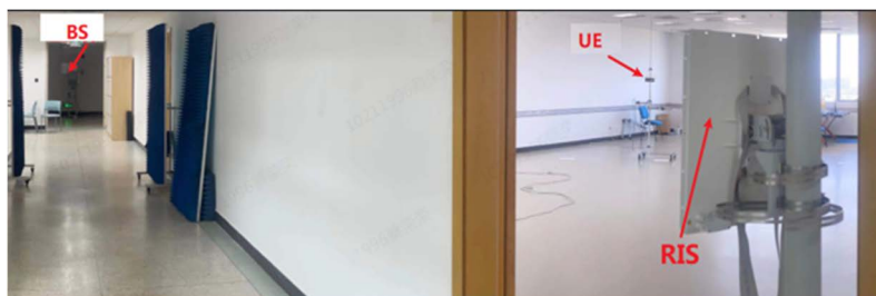
Figure 6.2-1: The setup for the indoor test [i.15]
