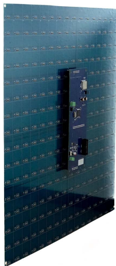
b) Back of the RIS and the controller
