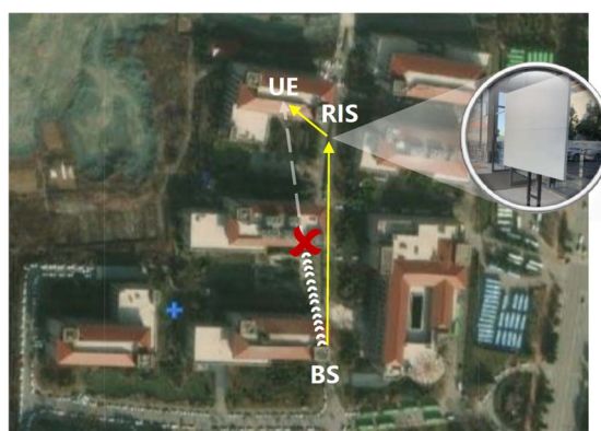
Figure 6.2-3: The setup for the O2I test at 2,6 GHz [i.15]
