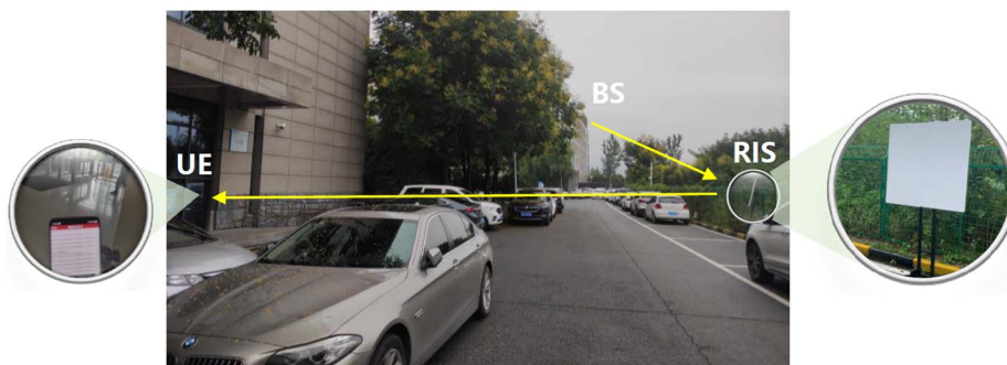
Figure 6.2-4: The setup for the O2I test at 4,9 GHz [i.15]
