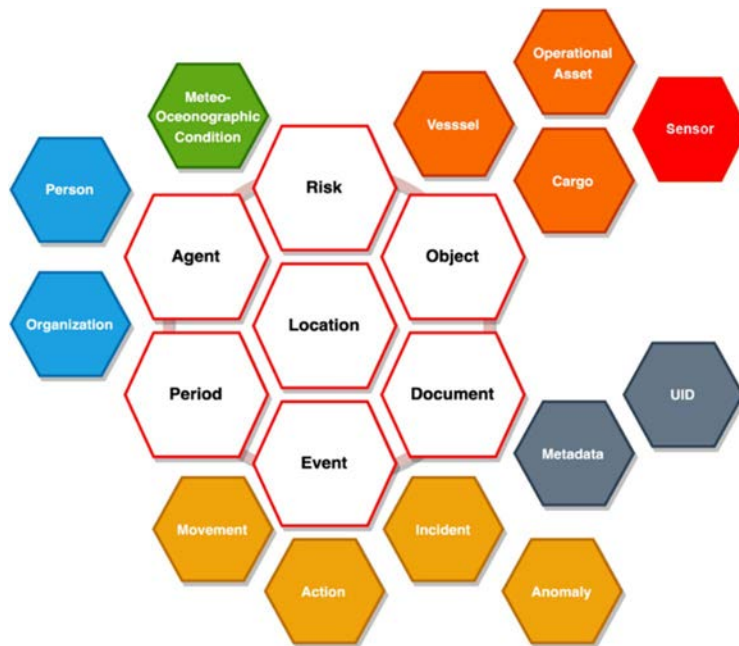
Figure 5.2-1: Enhancement of the CISE Information Model based on the maritime vocabulary extension
