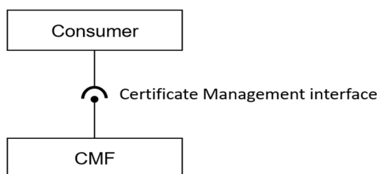
Figure 5.2.2.2.1-1: Exemplary illustration of CMF and its exposed certificate management interface
