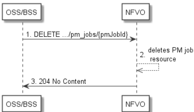
Figure 7.3.3-1: Flow of PM job deletion
