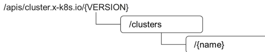
Figure 9.3-1: Resource URI structure of Cluster resource object for the CIS cluster fault management service interface
