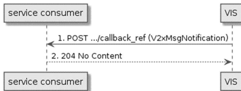
Figure 5.5.10.3-1: Flow of V2X message notification
