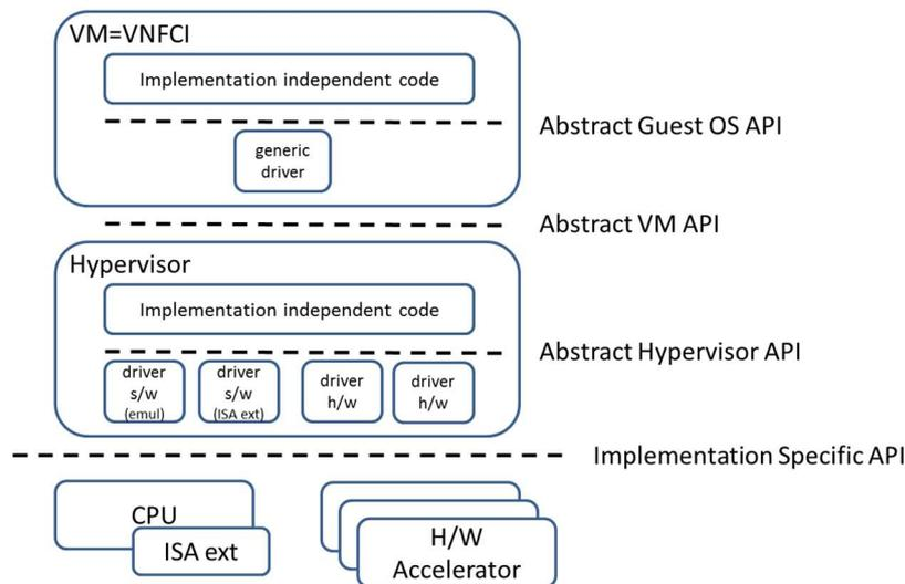
**Figure 4.0-1: NFV acceleration abstraction layer implemented within hypervisor as a disaggregated model**
