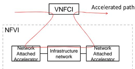
**Figure 5.2-2: Accelerator chaining**
