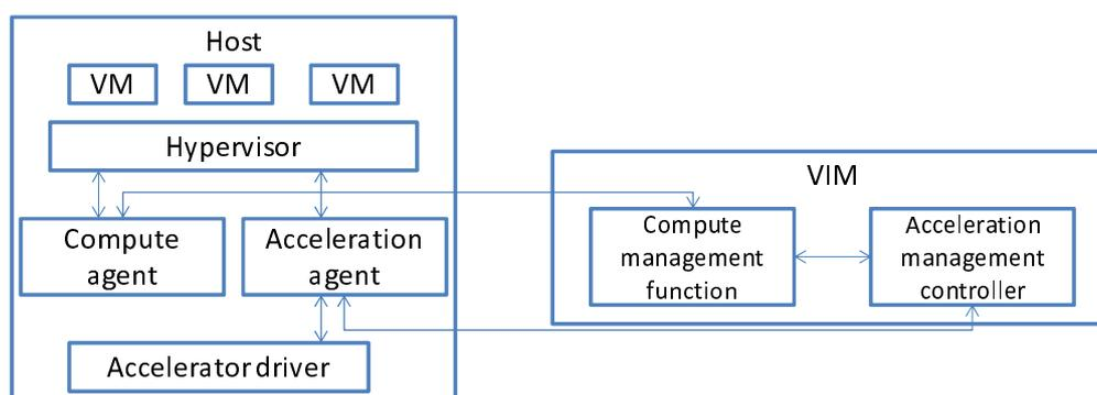
**Figure B.2.1-1: Acceleration management architecture example**
