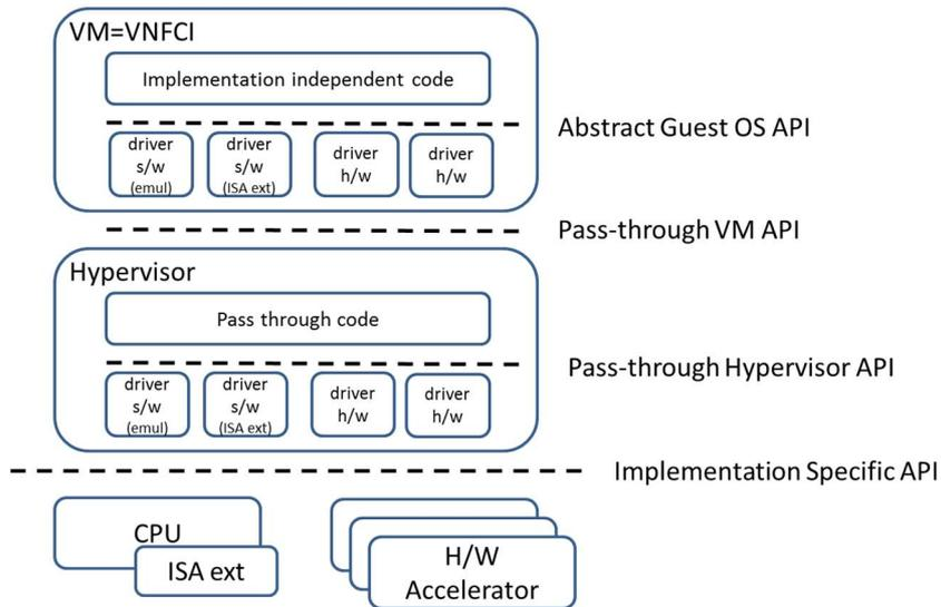
Figure 4.0-2: NFV acceleration abstraction layer implemented within VNF as an integrated model
