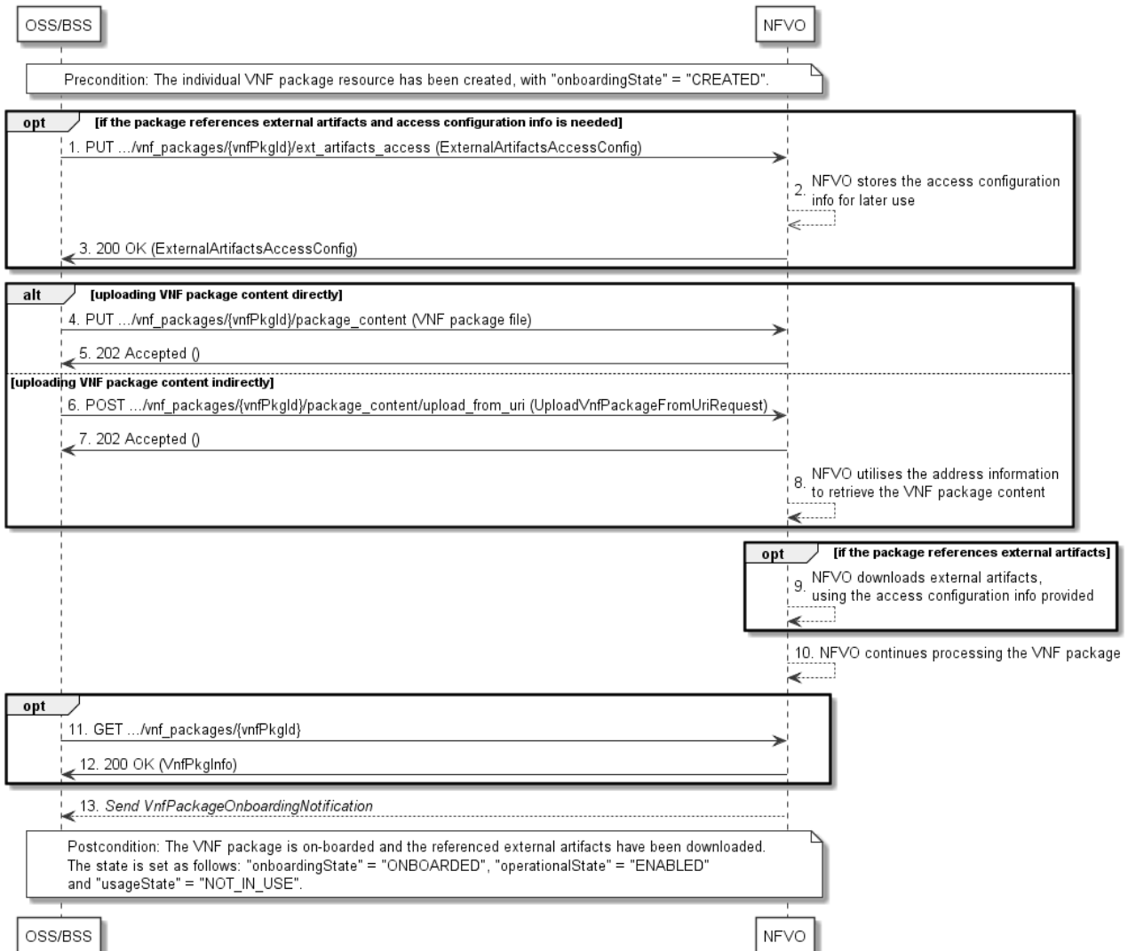
Figure 9.3.2-1: Flow of the uploading of VNF package content
