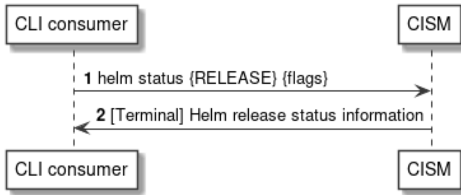
Figure 7.3.5-1: Flow of containerized workload information querying
