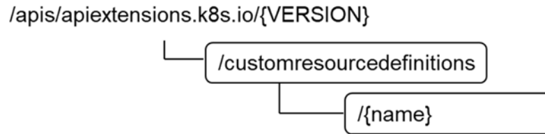
Figure 11.3-2: Resource URI structure of CustomResourceDefinition resource object for the OS container configuration management service interface
