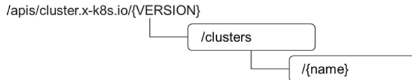
Figure 6.3-1: Resource URI structure of Cluster resource object for the CIS cluster lifecycle management service interface
