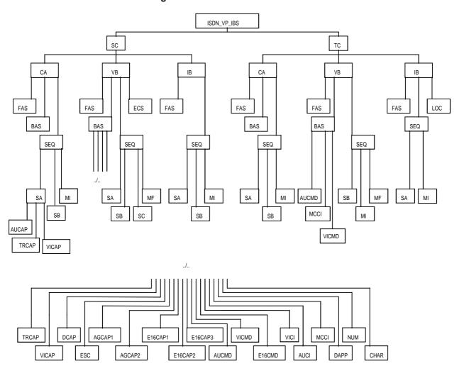
**Figure 1: Test Suite Structure**
