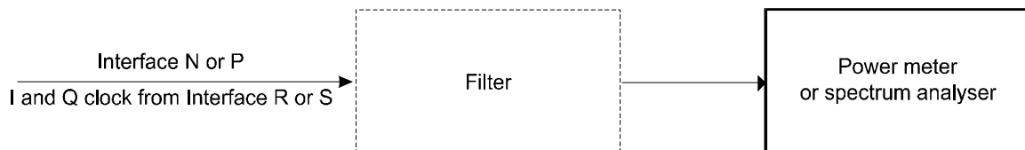
Figure B.7: Test set-up for RF/IF level measurement
