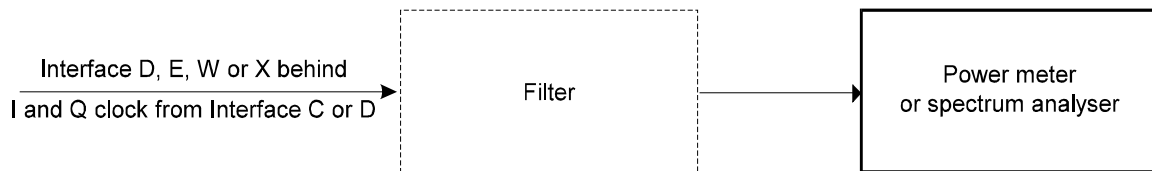
Figure E.14: Test set-up for out-of-service noise power measurement
