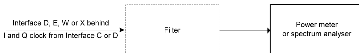
Figure E.13: Test set-up for RF/IF power measurement
