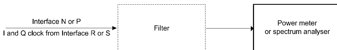
Figure B.8: Test set-up for out-of-service noise level measurement
