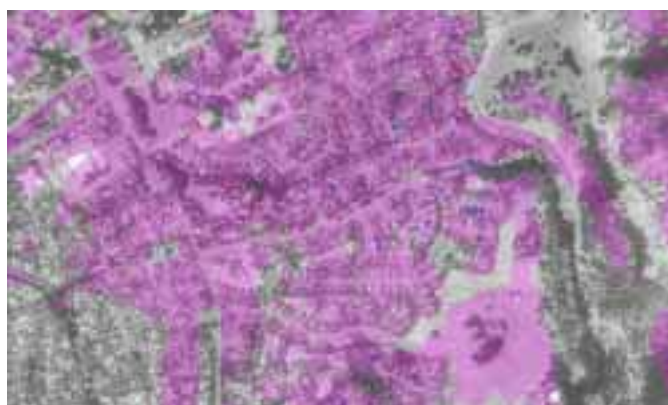
Figure B.5: Mesh Access Point node with 5 subscriber nodes coverage
