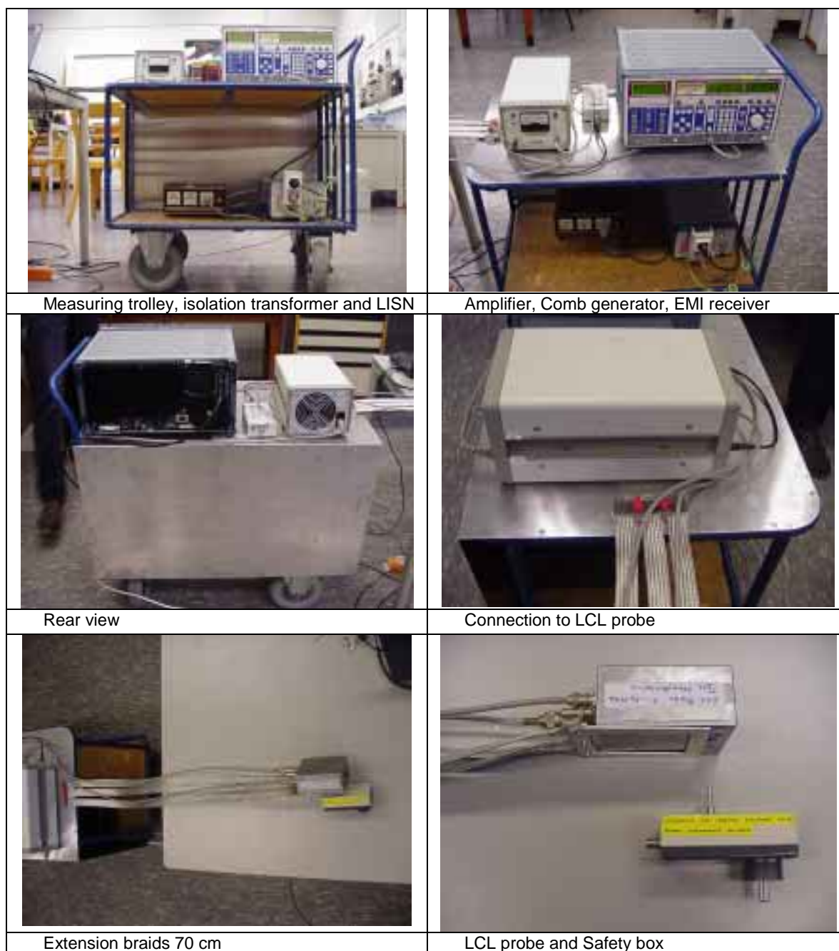
Figure 5.1: Measurement trolley with various test equipment
