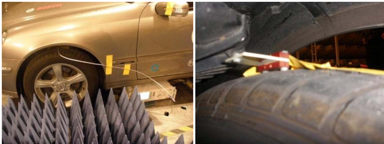
Figure 18: Car setup with antenna in the fender
