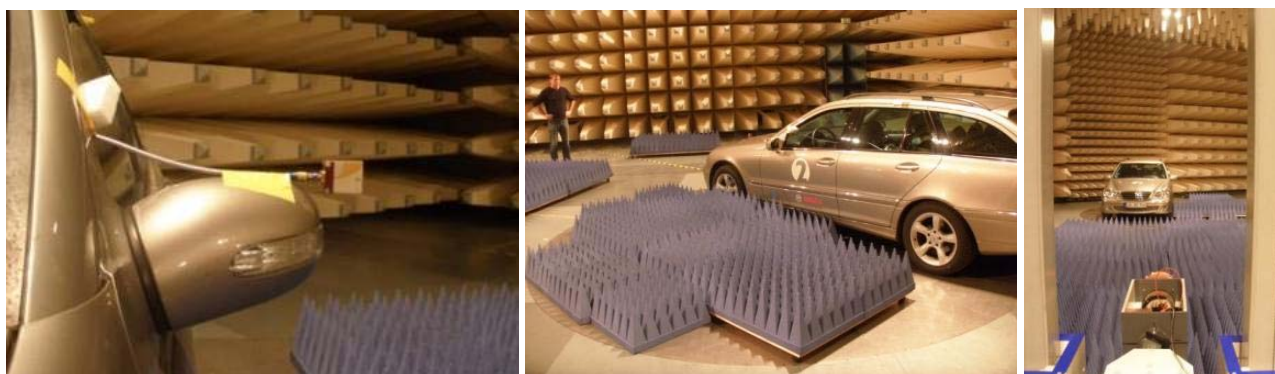
Figure 16: TX antenna on the side mirror
