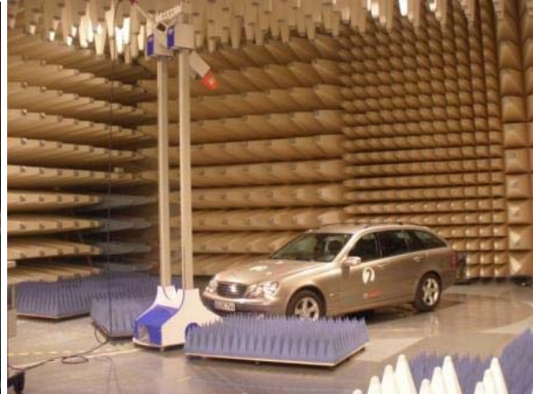
(b) RX antenna at 3m and 4m height (42°)
