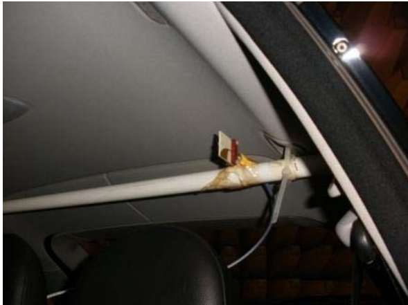
(a) TX antenna under the roof
