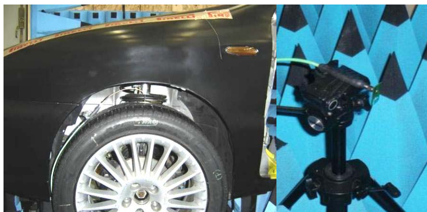
Figure C.28: UWB Antenna inside the tire (left) and standalone (right)
