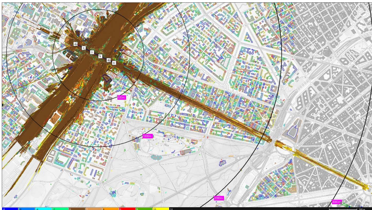
Figure A.16: Paris L1 - Difference of the received interference level in dB, for a Road-ITS antenna height variation between 1,5 m and 1,7 m, for Road-ITS EIRP of 33 dBm and a CBTC DSSS with 3 dB desensitization (Source: ©OpenStreetMap contributors - www.openstreetmap.org/copyright )
