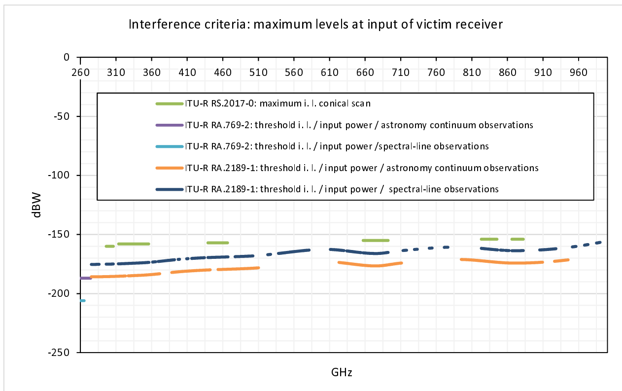
Figure 18: Harmful interference thresholds for satellite passive remote sensing and radio astronomy according to Recommendation ITU-R RS.2017-0 [i.12] and Report Recommendation ITU-R RA.2189-1 [i.5] in the frequency range from 260 GHz to 1 000 GHz
