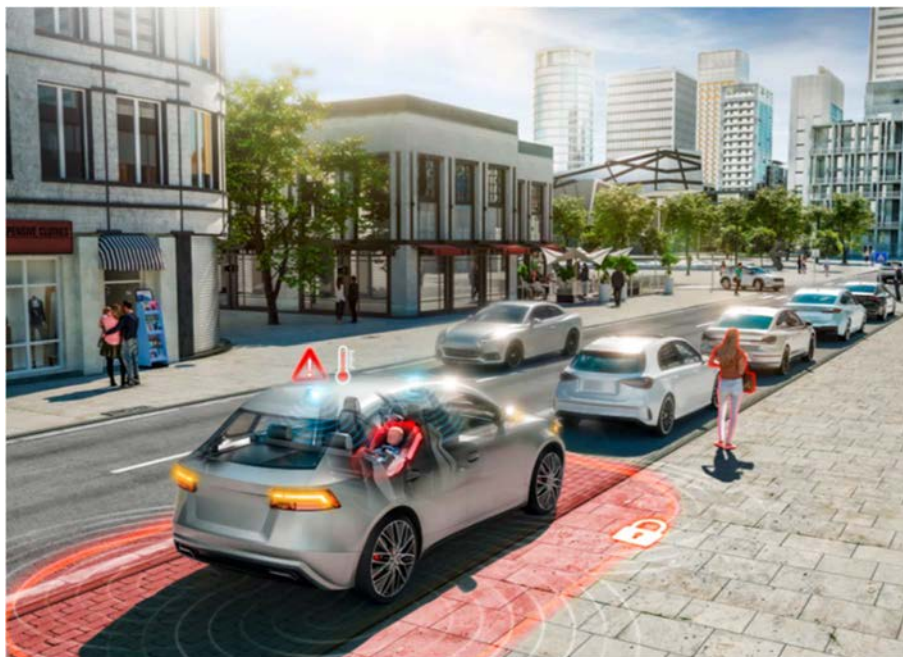
Figure 10: Child Presence Detection (CPD) application using UWB (copy pictures courtesy of AUMOVIO)
