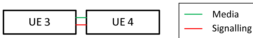
Figure2: Off-network architectural model for 5G inter-UE communication where no relay function is used
