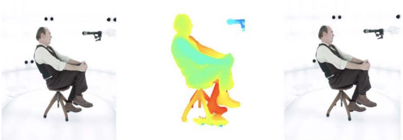
Figure 4.6.7-4: Example of a dense depth map calculated per frame for each stereo camera pair
