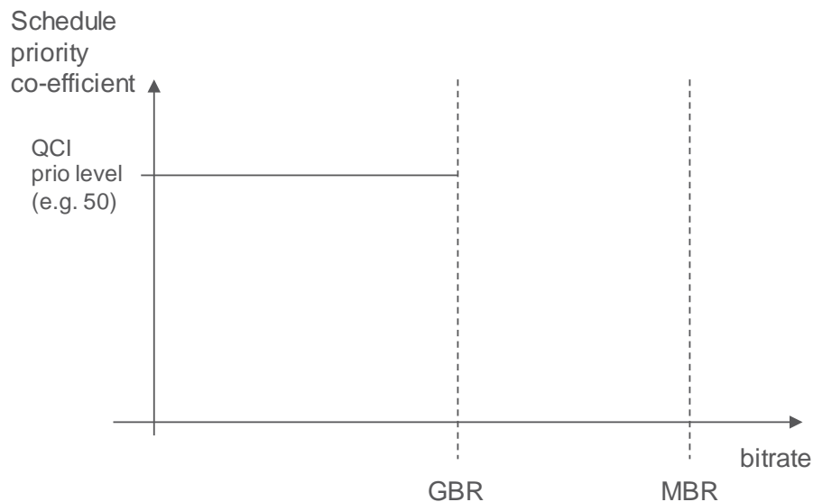
Figure 9.2.4-1: Today's prioritization: traffic gets priorities up to the GBR and is treated as best effort above GBR
