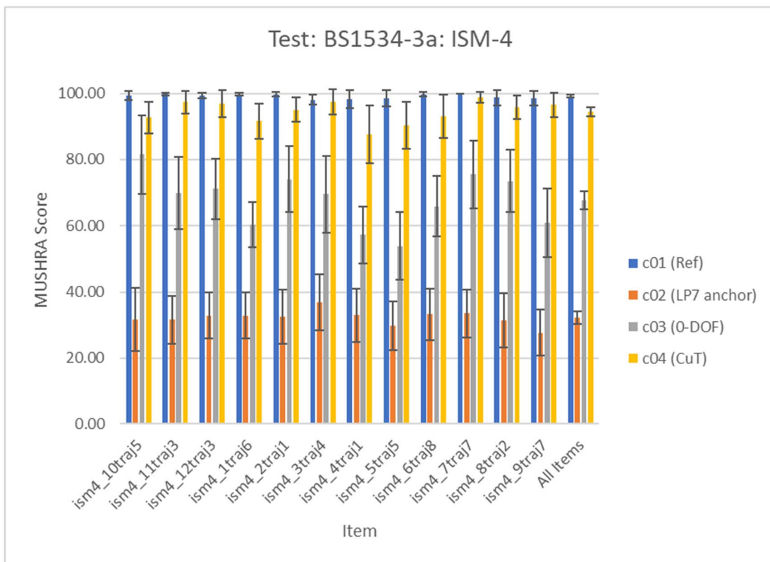
Figure 6.1-5: Results of BS1534-3a test for ISM-4 input audio
