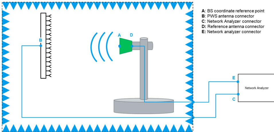
Figure 8.6-1: Path loss calibration in PWS, TX requirements
