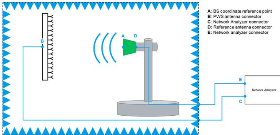
Figure 8.6-1: Path loss calibration in PWS, TX requirements
