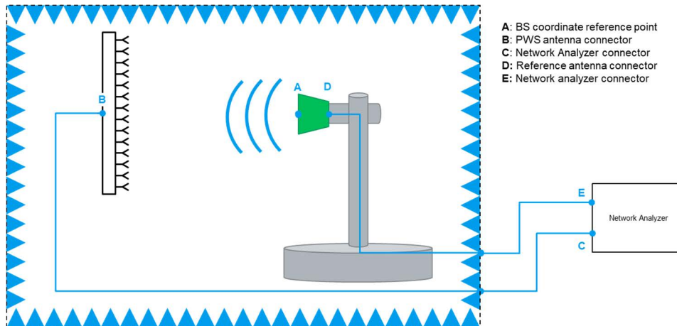
Figure 8.6-1: Path loss calibration in PWS, TX requirements
