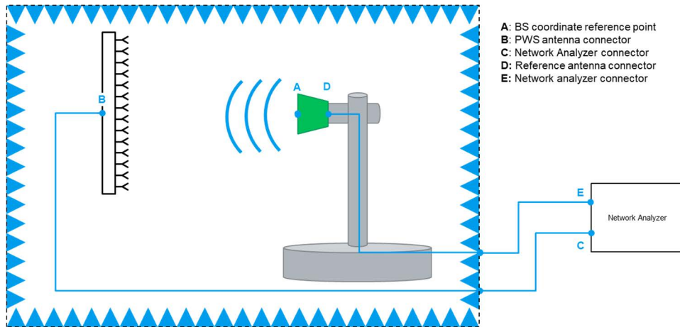
Figure 8.6-1: Path loss calibration in PWS, TX requirements
