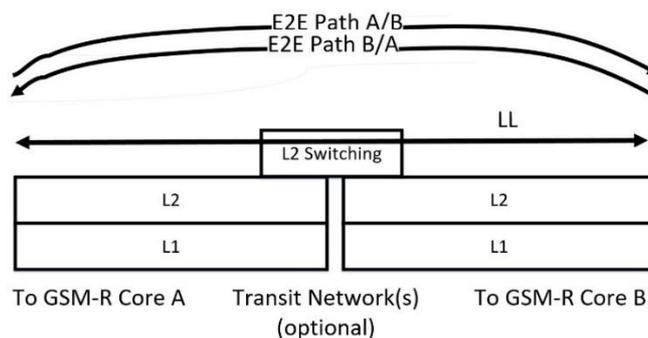
**Figure 6: E2E IP path, when being switched at transit**
