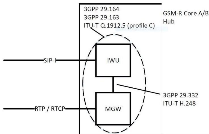
Figure 10: Major Standards for the handling of SIP-I and RTP/RTCP traffic at the edge of the network
