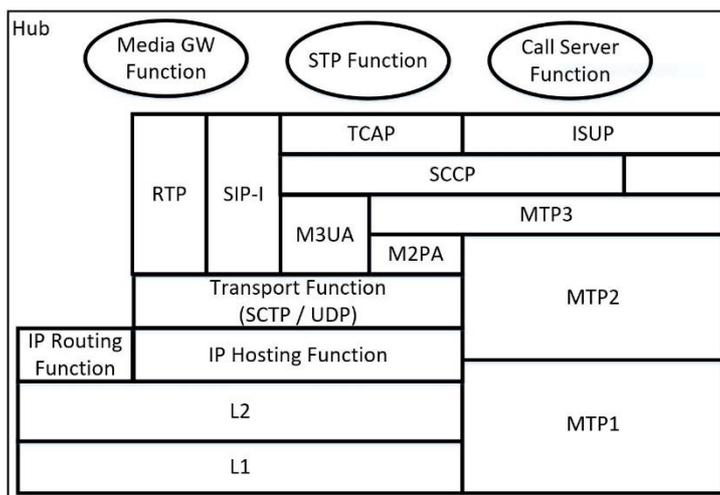
**Figure 2: Lower layer protocols and network functions of a hub during migration**
