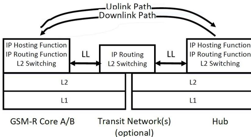
**Figure 5: UL/DL IP path, when being routed at transit**
