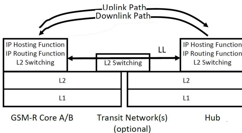
**Figure 4: UL/DL IP path, when being switched at transit**
