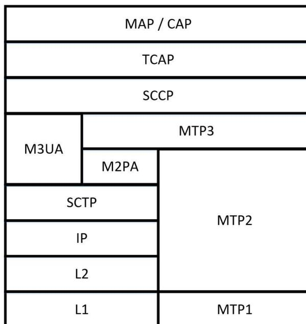
**Figure 13: Protocol stack for the interworking of SS7 traffic at the hub**
