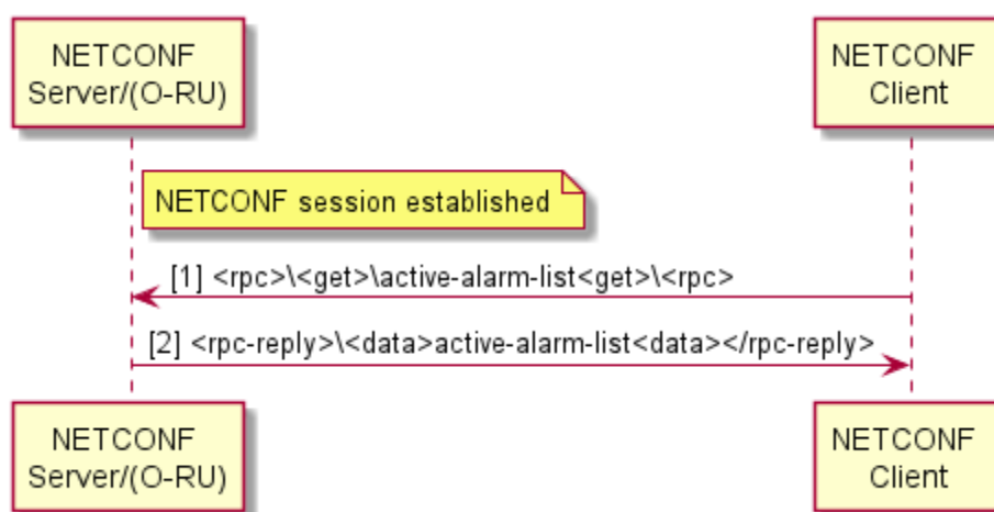
Figure 11.1-1: Read Active Alarms
