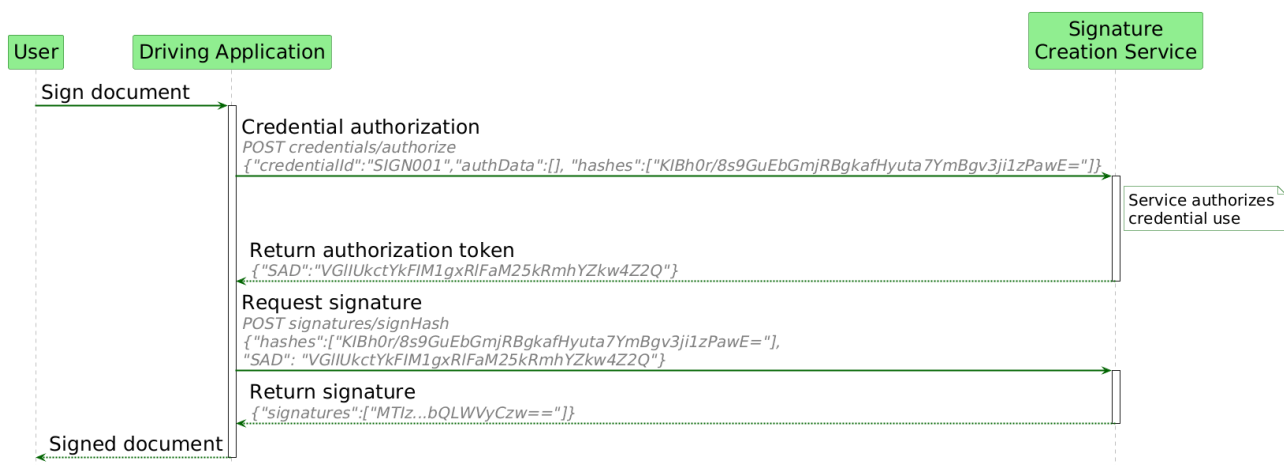
Figure 7: Remote hashes signature creation by using a signing credential whose usage is protected by authorization mechanisms managed by the signature creation service
