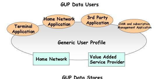
Figure 2: Illustration of the scope of 3GPP Generic User Profile
