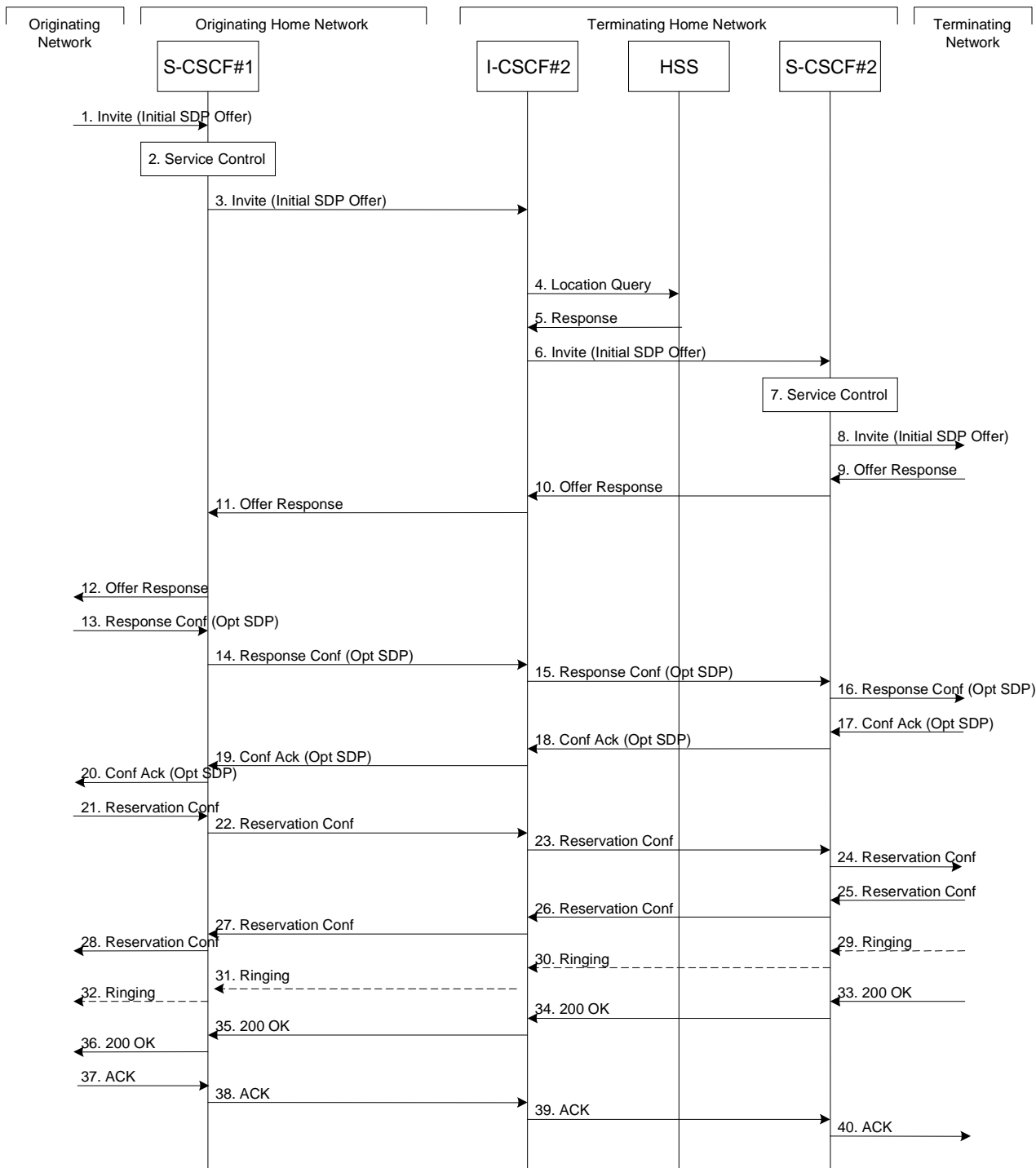
Figure 5.10: Serving to serving procedure - different operators
