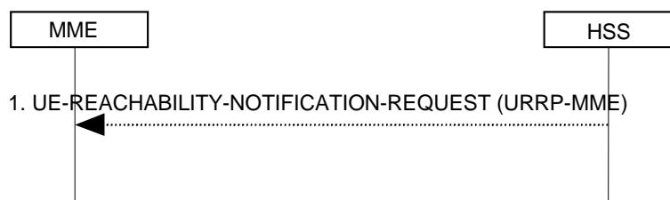
Figure 5.3.11.2-1: UE Reachability Notification Request Procedure
