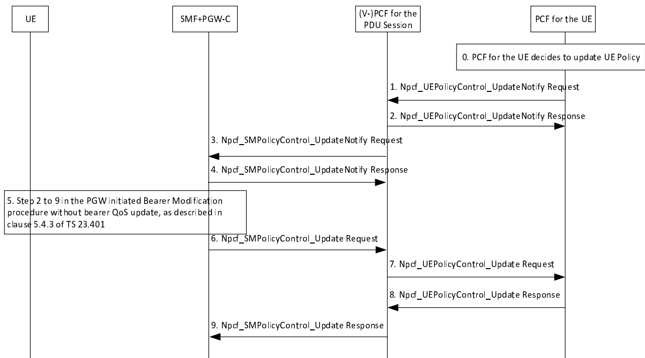
Figure 4.11.0a.2a.10-1: UE Policy Container delivery via EPS procedure
