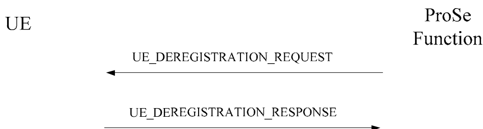
Figure 7.2.6.3.1.1: Network-initiated UE deregistration procedure
