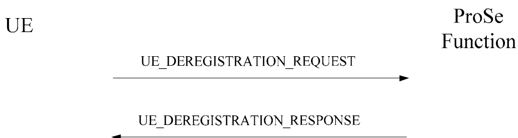
Figure 7.2.6.2.1.1: UE-initiated UE deregistration procedure
