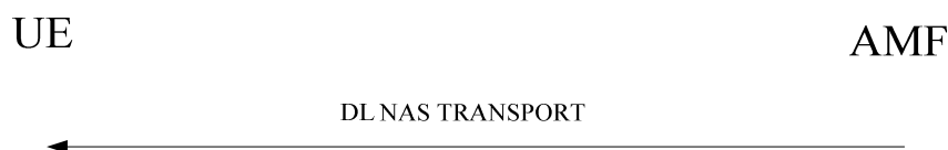
Figure 5.4.5.3.2.1: Network-initiated NAS transport procedure
