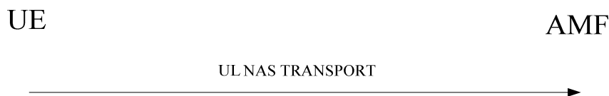
Figure 5.4.5.2.2.1: UE-initiated NAS transport procedure
