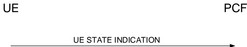
Figure D.2.2.2.1: UE-initiated UE state indication procedure
