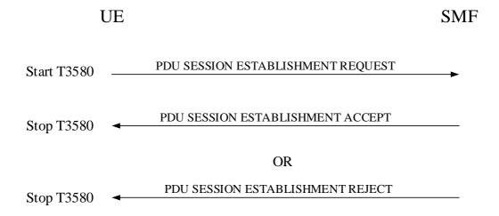
Figure 6.4.1.2.1: UE-requested PDU session establishment procedure
