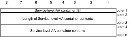
Figure 9.11.2.10.1: Service-level-AA container information element
