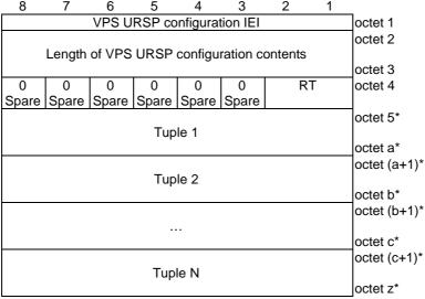
Figure D.6.8.1: VPS URSP configuration information element
