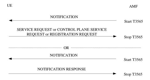
Figure 5.6.3.2.1: Notification procedure
