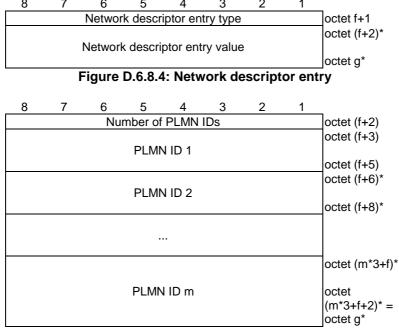
Figure D.6.8.5: Network descriptor entry value for network descriptor entry type set to "one or more VPLMNs"
