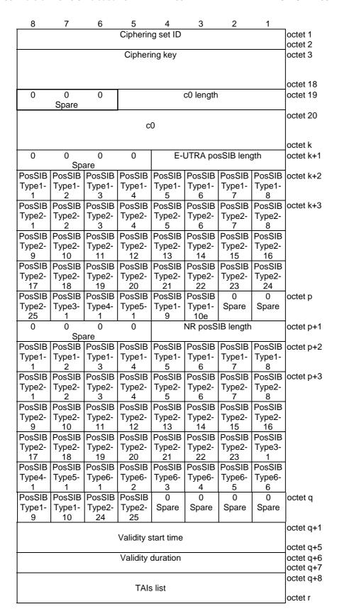
Figure 9.11.3.18C.2: Ciphering data set
