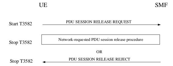
Figure 6.4.3.2.1: UE-requested PDU session release procedure
