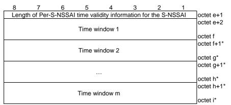
Figure 9.11.3.101.3: Per-S-NSSAI time validity information for the S-NSSAI
