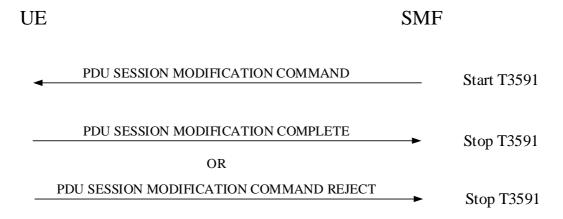
Figure 6.3.2.2.1: Network-requested PDU session modification procedure
