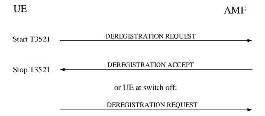
Figure 5.5.2.2.1.1: UE-initiated de-registration procedure
