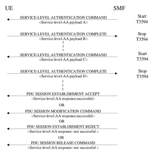
Figure 6.3.1A.1-1: Service-level authentication and authorization procedure
