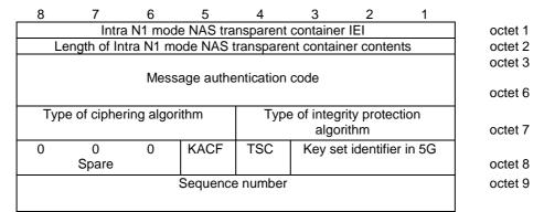
Figure 9.11.2.6.1: Intra N1 mode NAS transparent container information element
