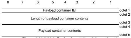
Figure 9.11.3.39.1: Payload container information element
