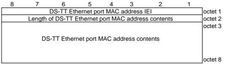
Figure 9.11.4.25.1: DS-TT Ethernet port MAC address information element
