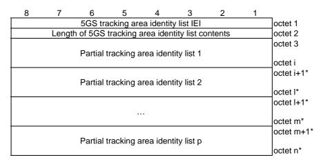
Figure 9.11.3.9.1: 5GS tracking area identity list information element
