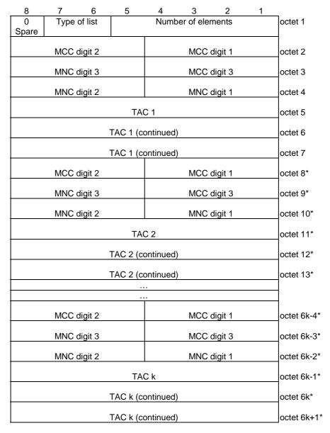
Figure 9.11.3.9.4: Partial tracking area identity list – type of list = "10"
