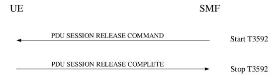
Figure 6.3.3.2.1: Network-requested PDU session release procedure
