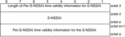
Figure 9.11.3.101.2: Per-S-NSSAI time validity information for S-NSSAI 1
