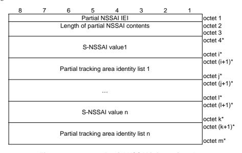
Figure 9.11.3.103.1: Partial NSSAI information element
