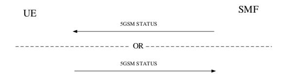
Figure 6.5.1.1: 5GSM status procedure
