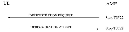
Figure 5.5.2.3.1.1: Network-initiated de-registration procedure
