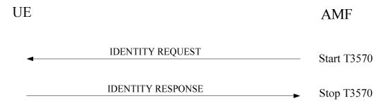
Figure 5.4.3.2.1: Identification procedure
