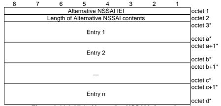
Figure 9.11.3.97.1: Alternative NSSAI information element
