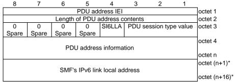
Figure 9.11.4.10.1: PDU address information element
