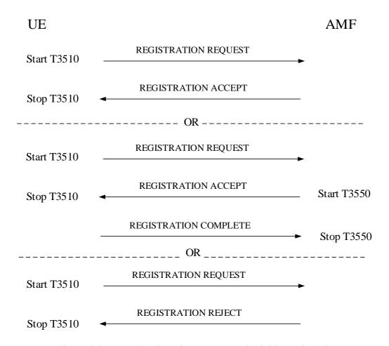
Figure 5.5.1.2.2.1: Registration procedure for initial registration
