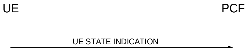
Figure D.2.2.2.1: UE-initiated UE state indication procedure
