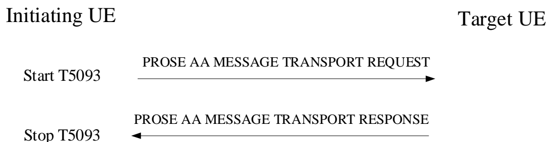
Figure 8.2.9.2.1: 5G ProSe AA message reliable transport procedure
