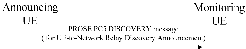
Figure 8.2.1.2.3.2.1: Monitoring UE procedure for UE-to-network relay discovery
