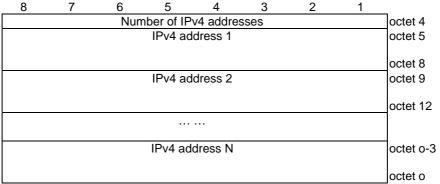
Figure 11.4.2.53.2: IPv4 address list
