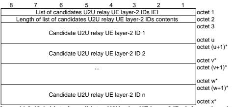
Figure 11.3.48.1: List of candidates U2U relay UE layer-2 IDs information element
