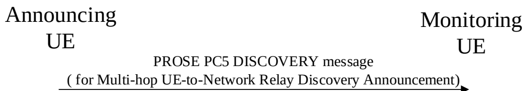
Figure 8b.2.1.2.2.3-1: ProSe intermediate UE-to-network relay UE procedure for multi-hop UE-to-network relay discovery initiation
