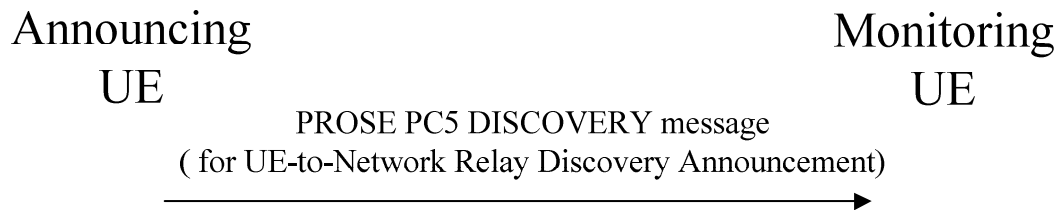
Figure 8.2.1.2.3.2.1: Monitoring UE procedure for UE-to-network relay discovery
