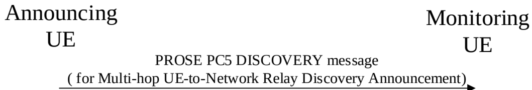
Figure 8b.2.1.2.2.2-1: ProSe multi-hop UE-to-network relay UE procedure for multi-hop UE-to-network relay discovery initiation
