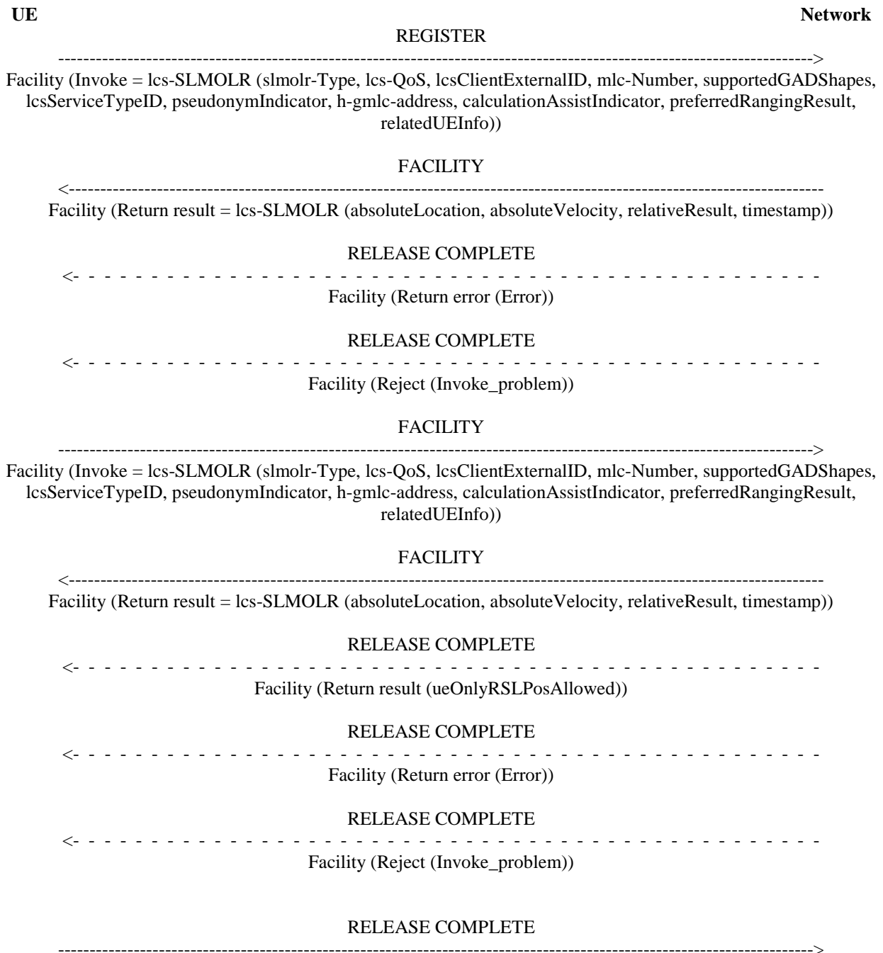
Figure 5.2.2.9.2-2: Multiple sidelink mobile originated location requests
