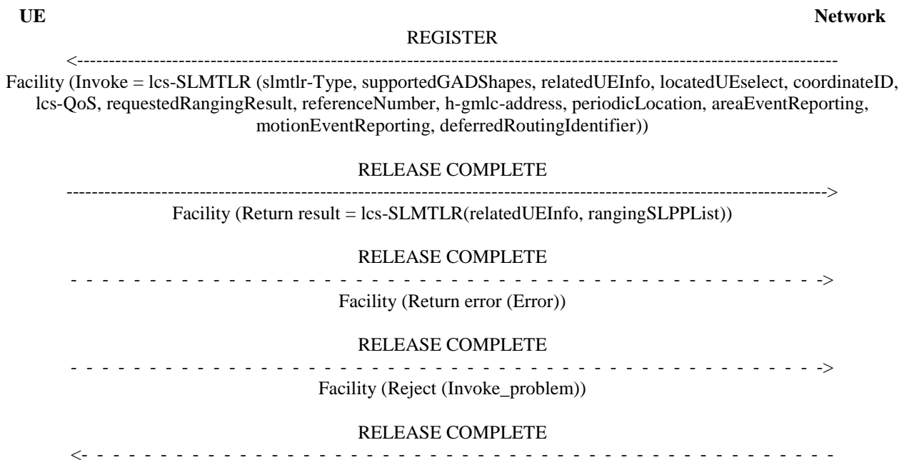
Figure 5.2.1.8.2.1: Sidelink mobile terminating location request procedure
