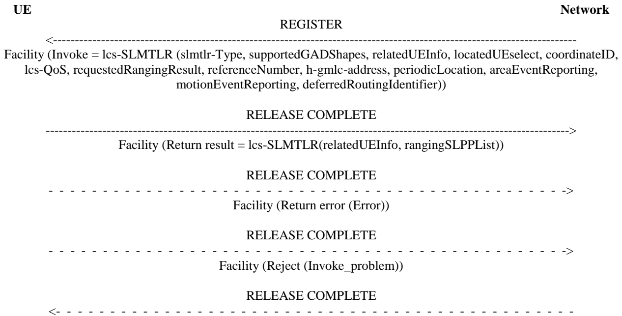
Figure 5.2.1.8.2.1: Sidelink mobile terminating location request procedure
