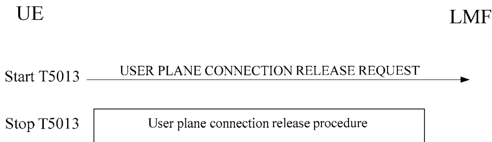
Figure 6.2.2.2.1: UE requested user plane connection release procedure
