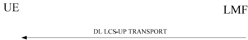
Figure 7.3.3.2.1: Downlink LCS-UP transport procedure
