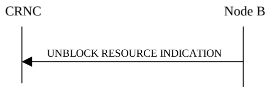
Figure 8: Unblock Resource procedure, Successful Operation
