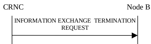
Figure 27O: Information Exchange Termination procedure, Successful Operation
