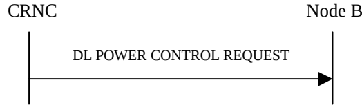
Figure 37: Downlink Power Control procedure, Successful Operation
