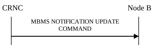
Figure 27Q: MBMS Notification Update procedure, Successful Operation
