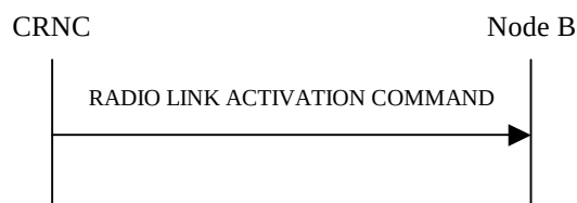
Figure 47D: Radio Link Activation procedure
