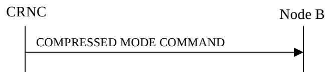
Figure 47: Compressed Mode Command procedure, Successful Operation
