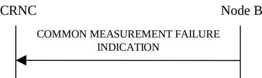
Figure 15: Common Measurement Failure procedure, Successful Operation
