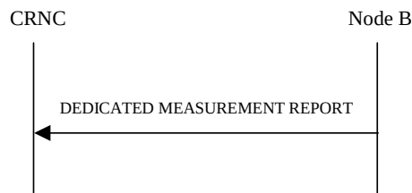
Figure 40: Dedicated Measurement Reporting procedure, Successful Operation
