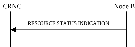
Figure 21: Resource Status Indication procedure, Successful Operation
