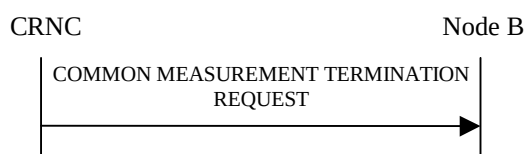
Figure 14: Common Measurement Termination procedure, Successful Operation
