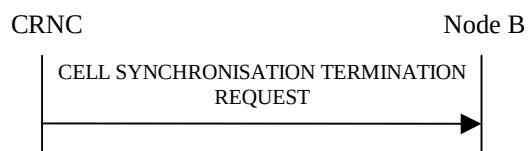
Figure 27H Cell Synchronisation Termination procedure, Successful Operation
