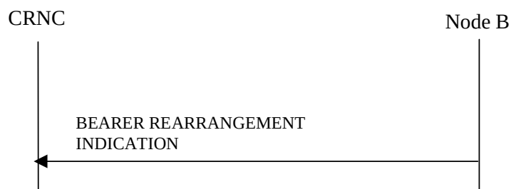
Figure 47C: Bearer Re-arrangement Indication, Successful Operation
