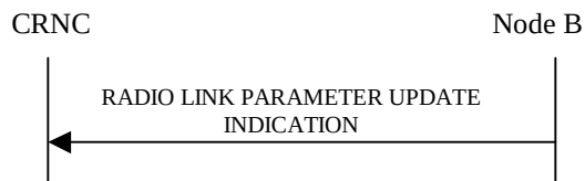
Figure 48: Radio Link Parameter Update Indication, Successful Operation
